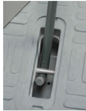
Recessed Lifting Pin with Cover
