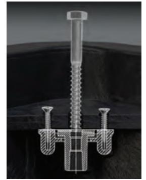
Non-Seizing Bolt System Allows Field Replacement
